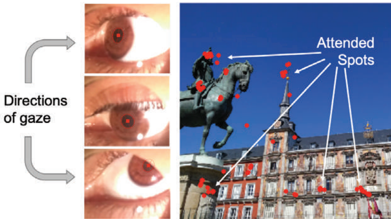
Figure 4 – Example of an eye tracking outcome. On the left are displayed pupil estimates for three different directions of gaze. On the right, superimposed to the image, several locations of visual attention. Adapted from [10].
