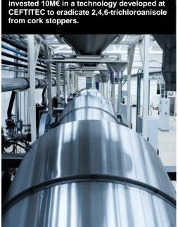
Under a contracted license with NOVA University Lisbon. Amorim Cork introduced in the production line of natural cork stoppers a technology developed at CEFITEC to
